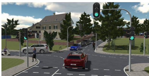
Vehicle under test (red) in urban environment* with SUMO surrounding vehicles, pedestrians, traffic lights
