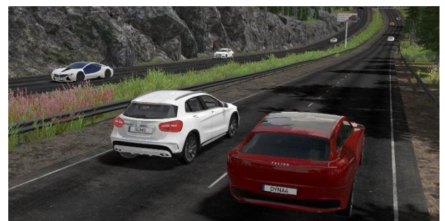
Rural environment: Vehicle under test (red) with SUMO traffic (white)
