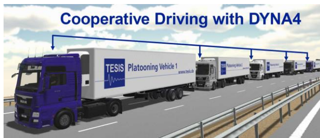
Five semi-trailer trucks under test in a platooning setup
