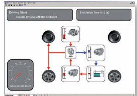
shows an example of the visualization of electric and mechanic energy flows for a driveline topology derived from the second-generation Toyota Prius.
