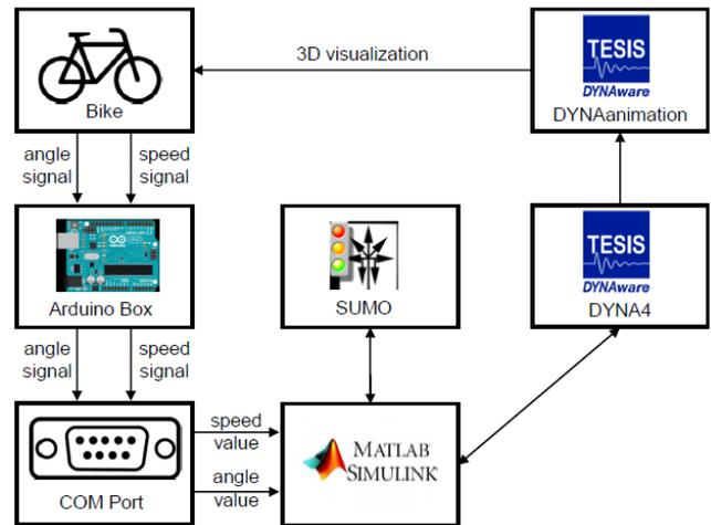
Starting with a physical bicycle that is connected to two identical sensors, magnetic rotary encoders, the information is read out via a microcontroller and sent via COM port to a processor. The incoming data is handled within a model (MATLAB Simulink) that connects the microscopic traffic flow simulation, via the software SUMO ([6], [7]) with the simulator software DYNA4 and DYNAanimation coming from the company TESIS.
