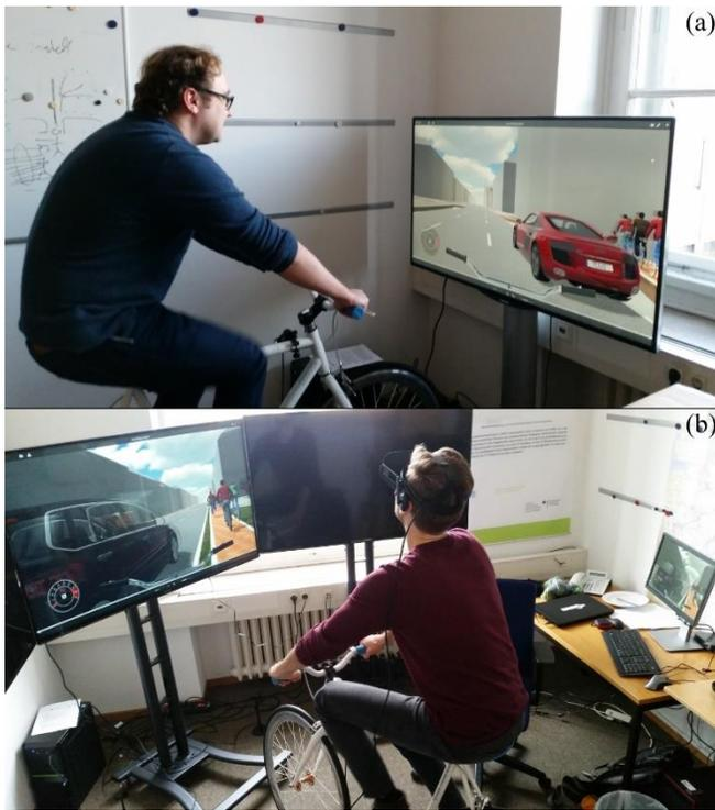
The option in Fig. 5b allows closed test conditions without observers being noticed by test subjects, since eyes and ears are visually and acoustically consumed by the simulation.
