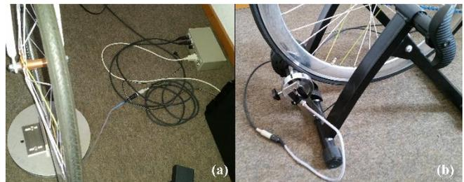
The animation of the simulator environment appears in connection with the sensor data coming from the two sensors on the steering plate (Fig. 2a) and the roller trainer (Fig. 2b) attached to the bicycle. As pictured in Figure 1, there is an additional software component for the visualization part: DYNAanimation. The simulator software and the software for microscopic traffic flow simulations have two kinds of
