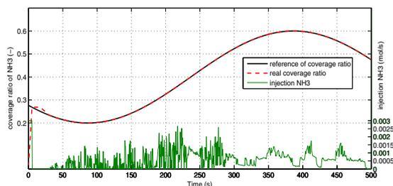
Fig. 8. Tracking response of sine input signal with low frequency
