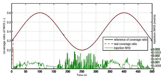
Fig. 7. Tracking response of sine input signal with high frequency
