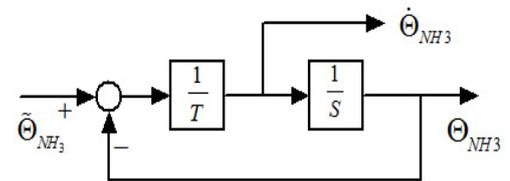
Fig. 2. First order filter for input shaping
