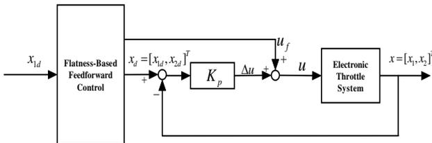
Fig. 3. Designed Feedforward-feedback Controller
