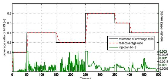
Fig. 9. Tracking response of step input signal
