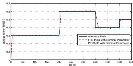
Fig. 10. Tracking response comparison: step input
