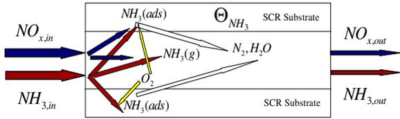
Fig. 1. Schematic presentation of the urea-SCR reactions
