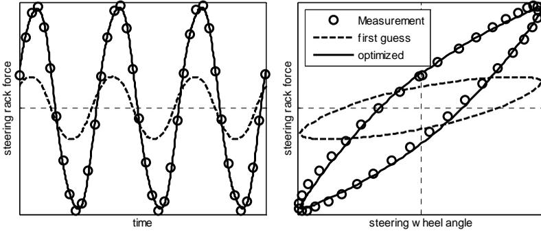
Figure 8: Sinusoidal steering input at standstill compared to full vehicle measurement
