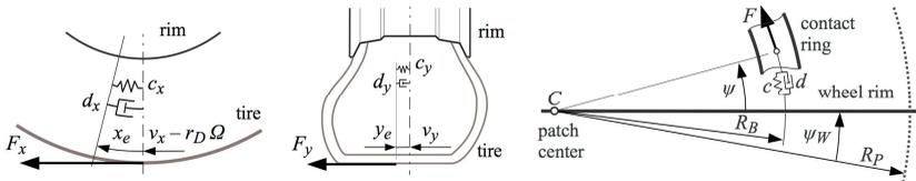
Figure 5: Tire deflection in the longitudinal, lateral and circumferential direction
