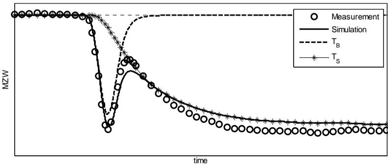
Figure 10: Self-aligning torque at a step response test on the tire test rig
