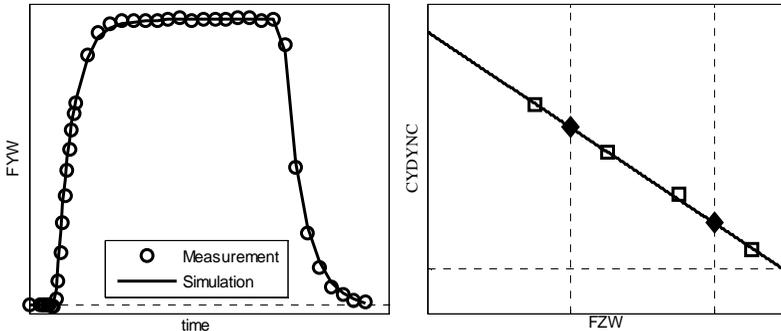
Figure 7: Lateral step response and parameter fitting (dynamic)
