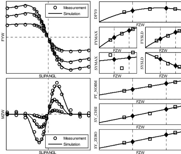
Figure 6: Fitting of lateral force and self-aligning torque parameters (quasi-static)
