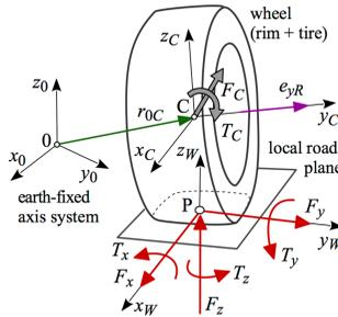
Figure 1: Axis systems, forces and torques
