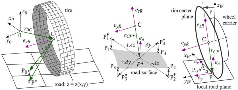
Figure 2: Contact geometry
