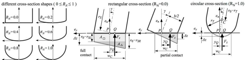
Figure 3: Different tire cross-section shapes and influence on the location of the contact points
