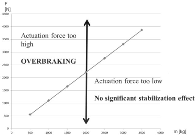
**Fig. 3.** Maximum permissible actuating force as a function of mass at  $\mu = 0.3$
