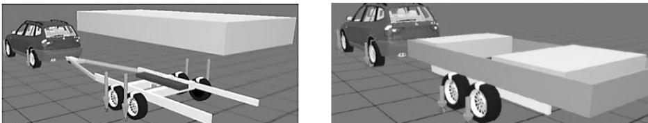
Fig. 8. Two different load variants in the simulation framework DYNA4 (left: abstracted sailboat trailer, right: high loader)
