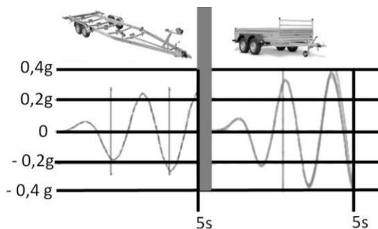
**Fig. 13.** Comparison of lateral acceleration during up-swing movement of a trailer with long (left) and short (right) drawbar length
