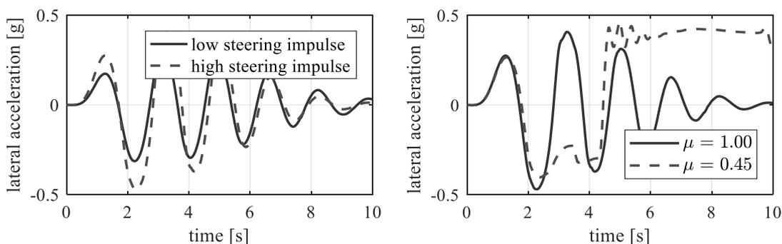
**Fig. 9.** Effect of different steering amplitudes (left figure) and different friction coefficients with the same trailer configuration and ATC intervention
