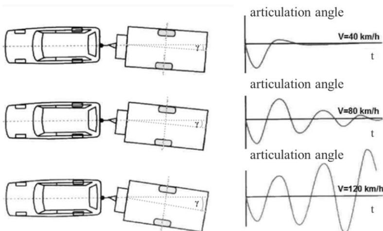
**Fig. 1.** Time course of the pendulum oscillation at different speeds without ATC intervention
