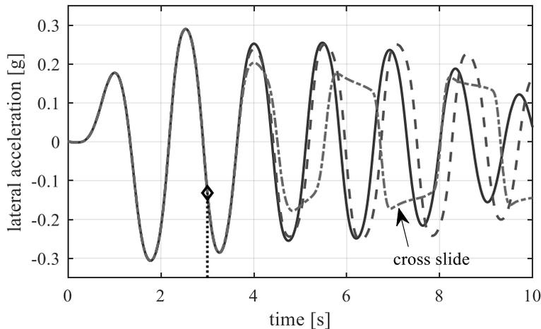
**Fig. 12.** Transverse movement identified by the lateral acceleration
