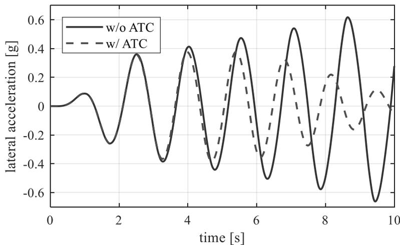
**Fig. 2.** Lateral acceleration with and without ATC intervention at supercritical speed
