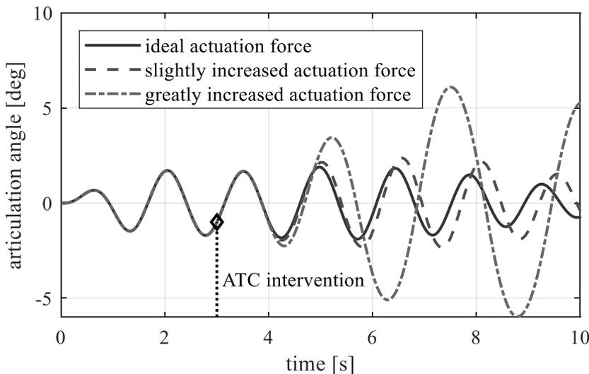
Fig. 11. Articulation angle for different actuation forces ( $\mu = 0,45$ ;  $m = 1250\text{kg}$ )
