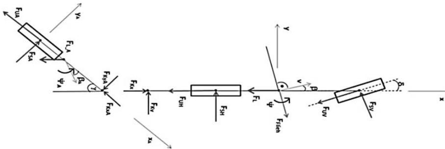
**Fig. 5.** Linear single track model of a car-trailer combination
