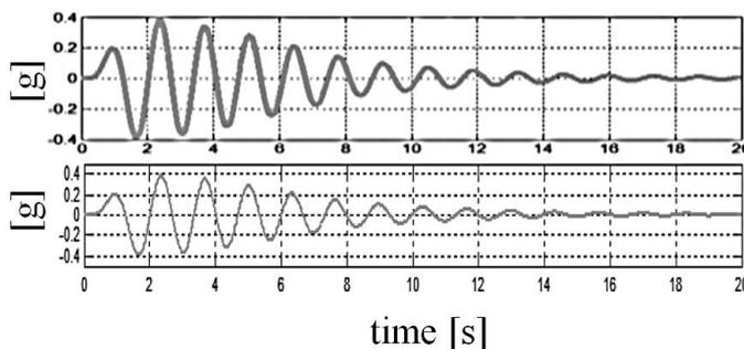
**Fig. 6.** Comparison of single-track model (top) and multi-body simulation (bottom) for a pendulum oscillation with ATC intervention at maximum amplitudes until 4 m/s<sup>2</sup>.
